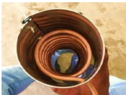
Figure 5: Inner view of the Heat exchanger
